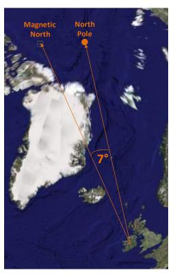
Technically there is another north called grid north. Grid north comes from the national grid which is a grid of  $5x5 = 25 \ 100 \ \text{Km}$  squares over Ireland. Obviously the north pointing edges are parallel and therefore cannot all point directly to true north but the difference is so slight we can (up to about 1°) take it that True and Grid north's are approximately equal.
